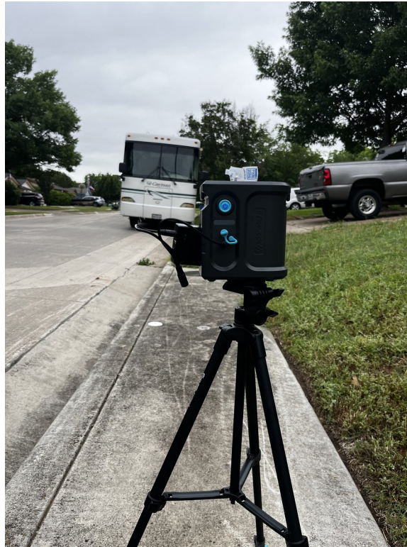
Photo 1: Outdoor air sampling station — spore trap cassette mounted on tripod at the property exterior. Sample 1 (outdoor baseline control).
